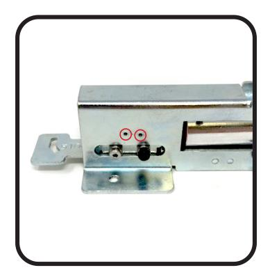
2. Using (2) Philips Screws and (2) Plastic Washers provided, mount Switch to Motor Assembly, Switch Arm should be facing down and rest on the Black Allen Screw, wires will run to rear of Motor.
